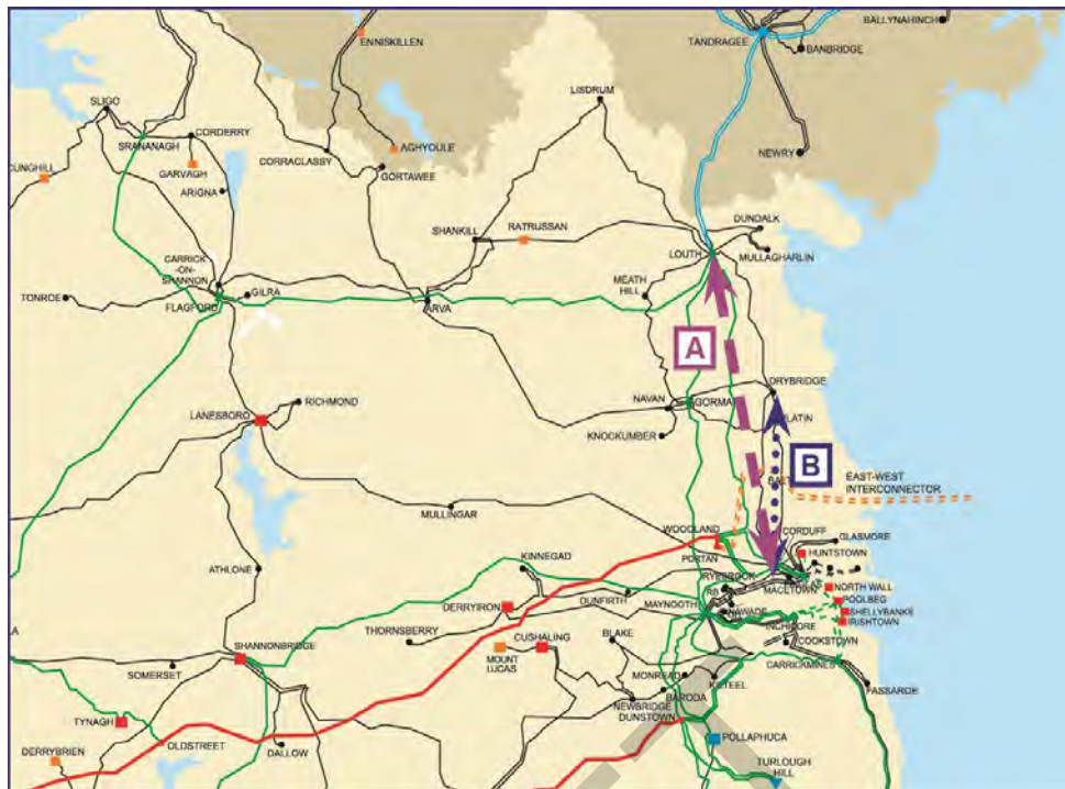
Figure 5.4: Strategic Alternatives for Transmission Reinforcement in the North-East
