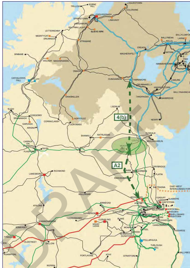
Figure 5.6: Opportunity for Strategic Linkage Between the Second Interconnector Project Option 4(b) and Transmission Reinforcement in the North-East Project Option A2 – at a Location along the Existing Flagford-Louth 220 kV Circuit
